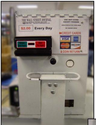
Using the price plate or template provided, use a punch to mark the placement of the holes to be drilled for installation of the card reader. Remove the price plate. Do not drill through the price plate. Use a 5/32" drill bit for the two small holes and a 7/16" drill bit for the large hole.
