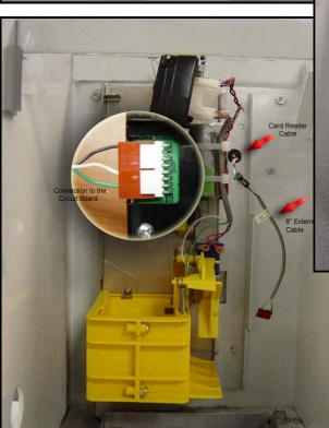
If this installation is for an ST-810, plug the card reader cable connector into the header on the reader body as shown below for the K-80.
