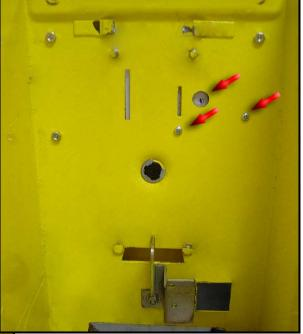
Put the card reader cable through the large hole from the front of the rack.
