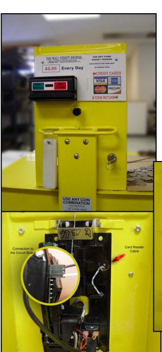
Using the price plate or template provided, use a punch to mark the placement of the holes to be drilled for installation of the card reader. Remove the price plate. Do not drill through the price plate. Use a 5/32" drill bit for the two small holes and a 7/16" drill bit for the large hole.
