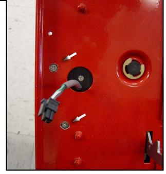
Put the card reader cable through the large hole from the front of the rack. Put
